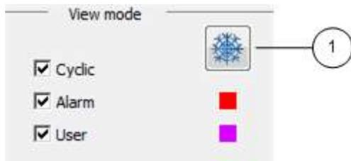
You can fetch needed waterfall (cyclic) curves, automatically saved alarm curves and curves you have stored yourself and display them all on screen. By default, waterfall curves are displayed when the analysis tool is launched.
