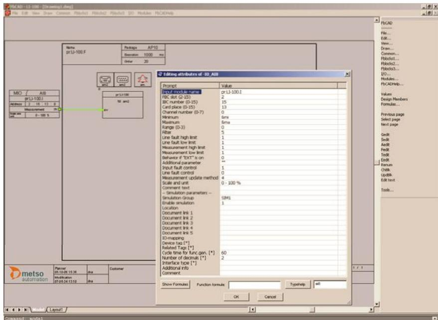
ACNI/O engineering in Function Block CAD engineering tool
