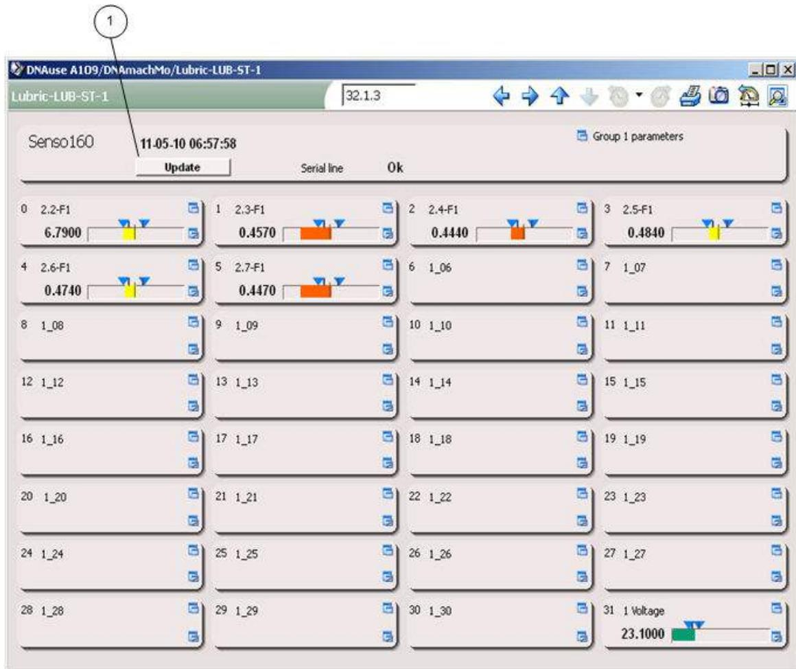
1. Manual update of station measuring results: reads station measurement values through a serial interface and updates results on screen.
