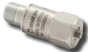
RVT/TT-125 is an industrial accelerometer with internal temperature sensor. Dual output sensor is an optimal solution for condition monitoring applications that utilize both vibration and temperature measurements.
