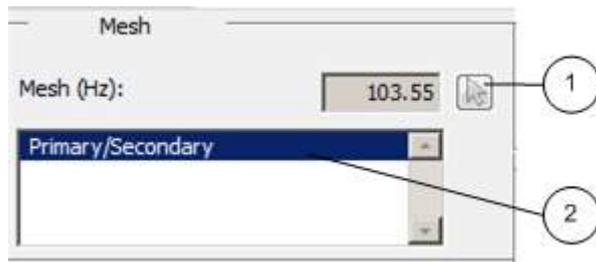
1. The first marker will be set to the gearmesh frequency on the spectrum by pressing the cursor button.
