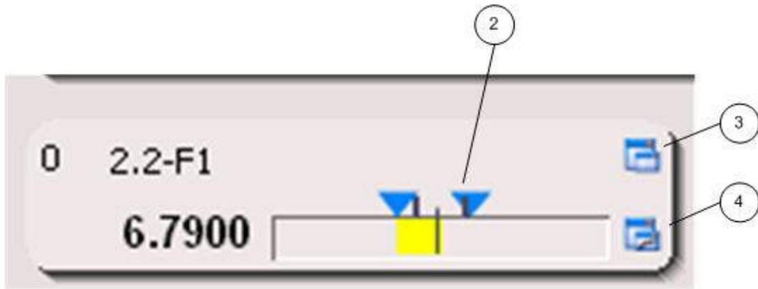
2. Lubrication channel measurement value as a number value and bar. The line in the middle of the bar indicates lubrication flow setting value. Bar color indicates alarm status (green: normal, yellow: warning, orange: alarm, red: zero flow alarm). The lines above the bar show warning limits and the triangles point to alarm limits (upper and lower limits).
