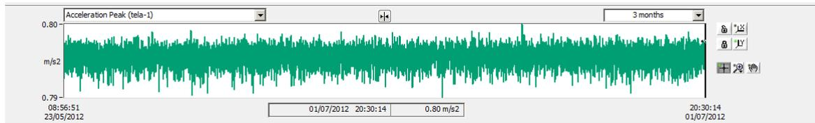
You can browse machine trends by selecting a trend from the drop-down list and fetch trend point curves by dragging the cursor in the trend view. The same scaling and zooming functions are available as in the spectrum window. You can also select the length of the trend from the drop-down list.
