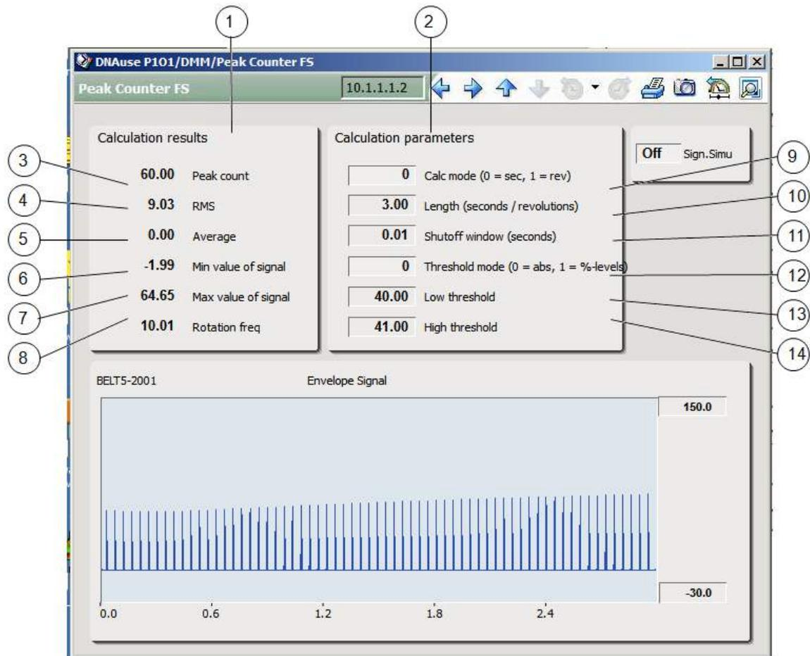
1. Results of internal calculations of the block used in PeakCount calculation.
