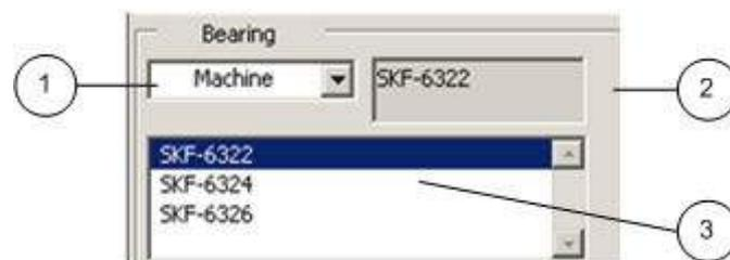
1. Bearing comparison. You can compare different bearing types by choosing either *Machine* or *All*. With the selection *Machine*, all bearings of the selected machine structure are displayed. With the *All* selection, all bearings in the component database are displayed.
