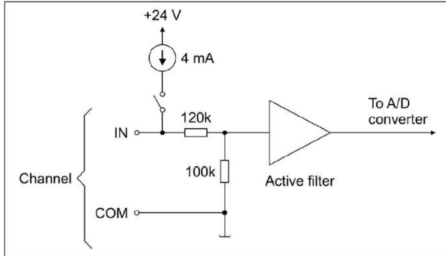
For the field cable connector of an AIF8V unit, the connection order for signals is as follows:
