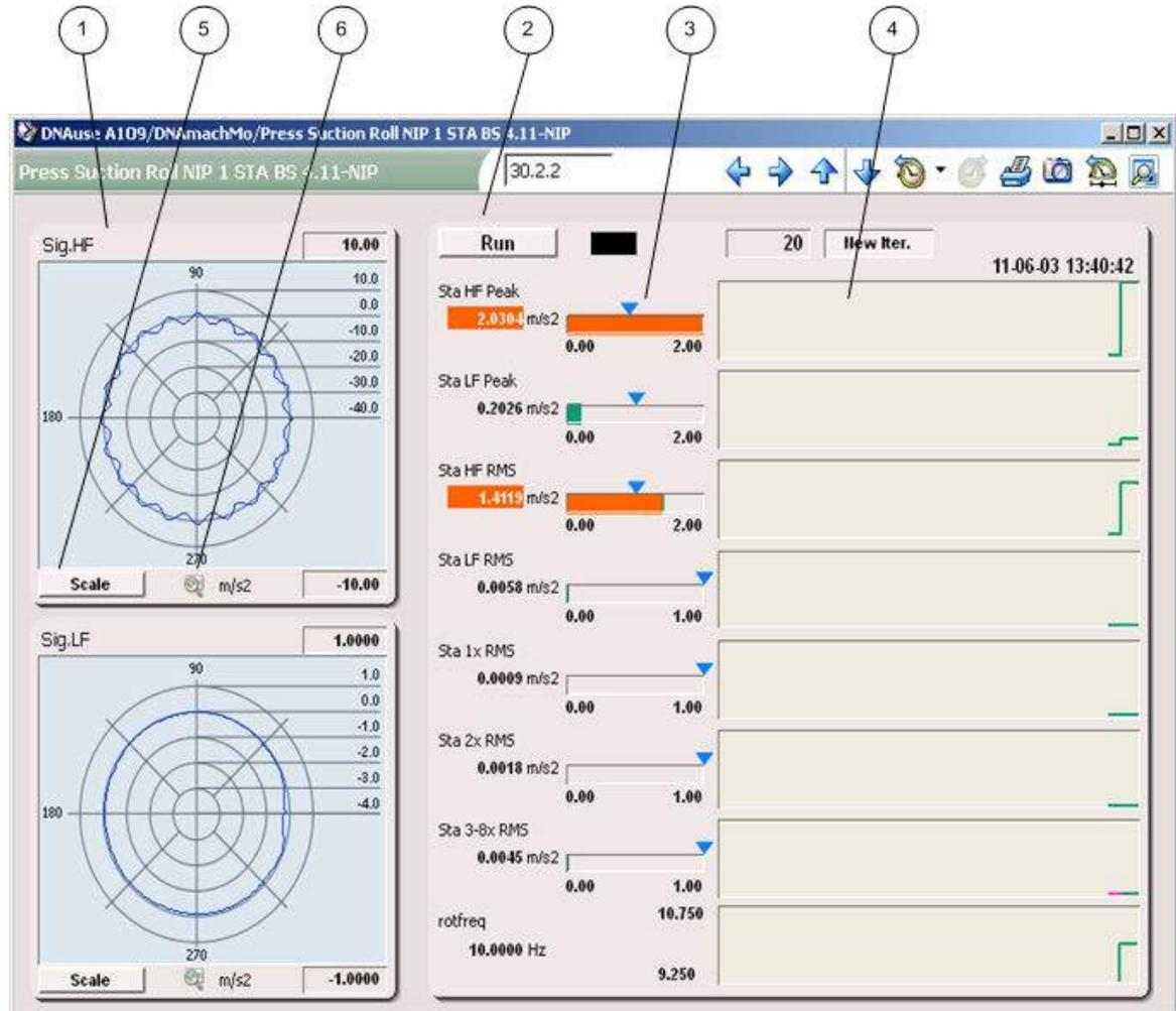
1. One-rotation-long STA vector in circle coordinates. High-frequency STA vector in the upper picture, low-frequency STA vector in the lower picture.
