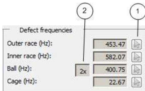
1. The cursor can be moved to the frequency of bearing defect frequencies and frequency multiplier by pressing the cursor button.
