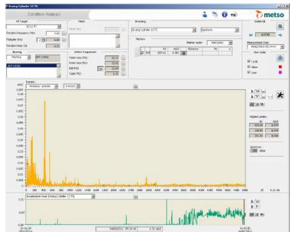
Layered user interface from overall view into detailed analysis tools suits both for operator's and predictive maintenance person's use.
