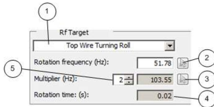
1. Point selection of rotation frequency. Points can be inserted with the Machine Structure Editor that is accessed by selecting *Modify* from the drop-down list.
