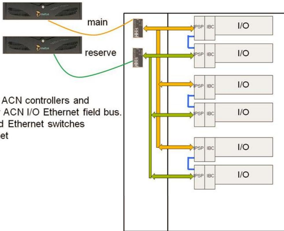
Redundant ACN controllers and twisted pair ACN I/O Ethernet field bus. Unmanaged Ethernet switches in I/O cabinet
